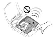
2 Press and hold down the ON/OFF button for 2 seconds to turn off the defibrillator and save battery power.
