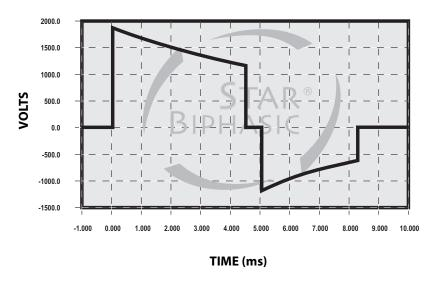
The Biphasic Truncated Exponential (BTE) waveform uses variable energy. The actual energy delivered will vary with the patient's impedance and the device will deliver a shock when impedance is between 25-180 Ohms. Energy will be delivered at three different levels referred to as ultra-low variable energy, low variable energy, and high variable energy as shown in the waveform tables on the following pages.
