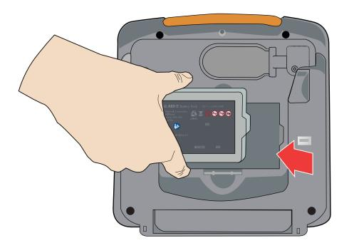
Remove the AED 3 battery from the shipping container. Hold the battery by the side tabs with the label facing out. Insert the battery into the back of the AED until it clicks into place, lining up the notch on the end of the battery to the corresponding shape in the battery well.
