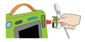
Plug the CPR Uni-padz cable connector into the AED 3 electrode port.
