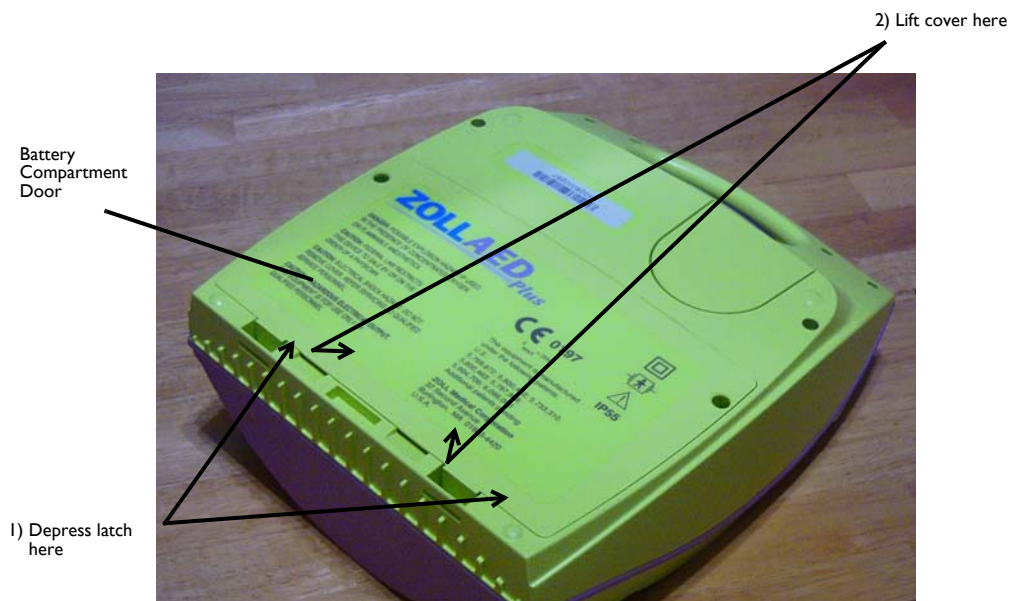
Figure 7: Removing the Battery Compartment Door
